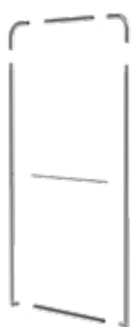
Add the central reinforcement and connect all the tubes with the help of the marking system
